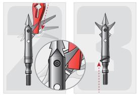
Insert wedge tool between blade and deployment arm (as shown). Return exposed blade into ferrule.
