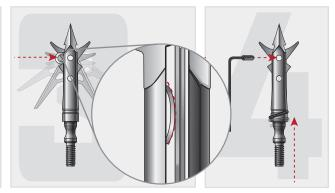
Rotate blades into the closed position. Install wave washer into ferrule as shown. Washer must be positioned between ferrule and blade.\*
