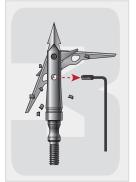
To return to hunting mode, remove practice mode screw, inspect the blades for damage, and remove any target debris.
